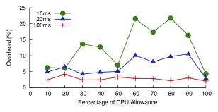
Figure 7: Overhead of CPU limiting which Fence inflicts on a CPU-intensive benchmark, at different polling rates.
