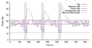
Figure 8: Fence restricts a benchmark's power draw using a simple token-bucket high-level policy [75]. *Tap* is the longterm power target; *reserve rate* the maximum currently allowed power. Benchmark idles in shaded regions.
